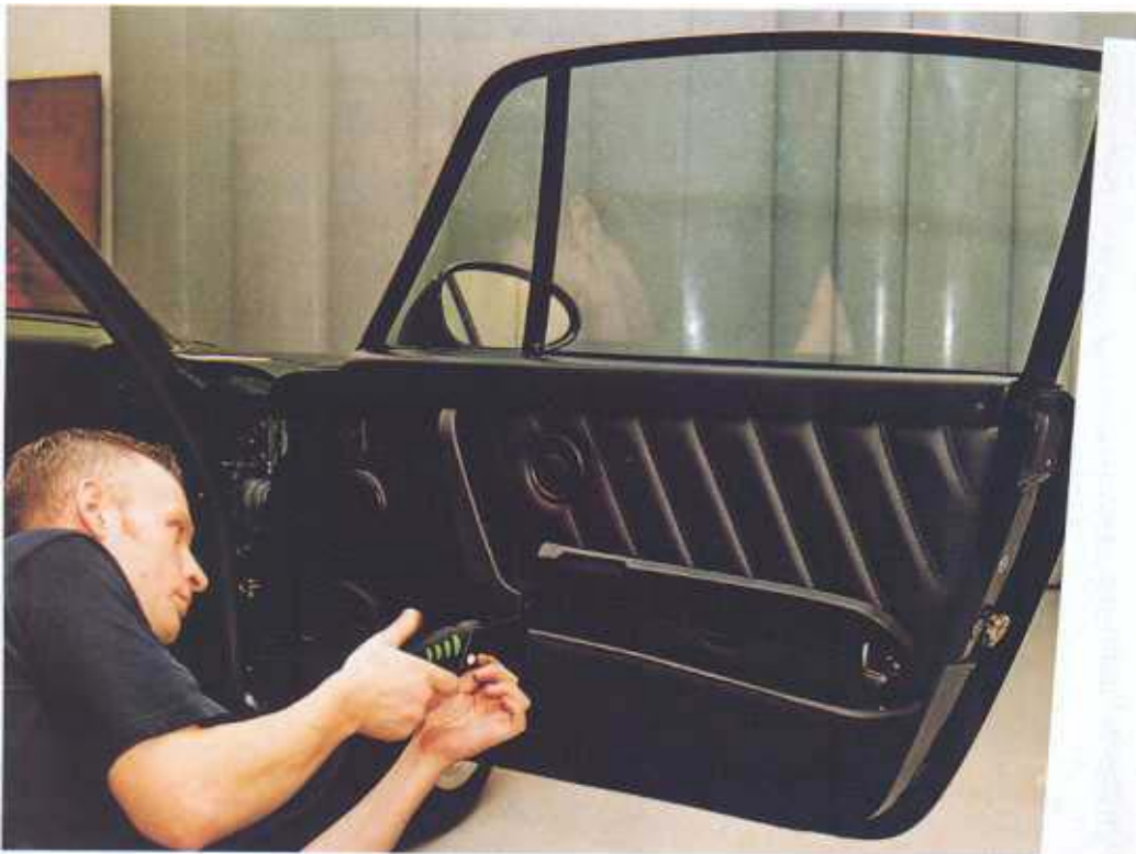
Replacing door furniture in our 911 takes time (above), although it's all screws, unlike the clips found in new cars. Entire job took about 10 hours start to finish
