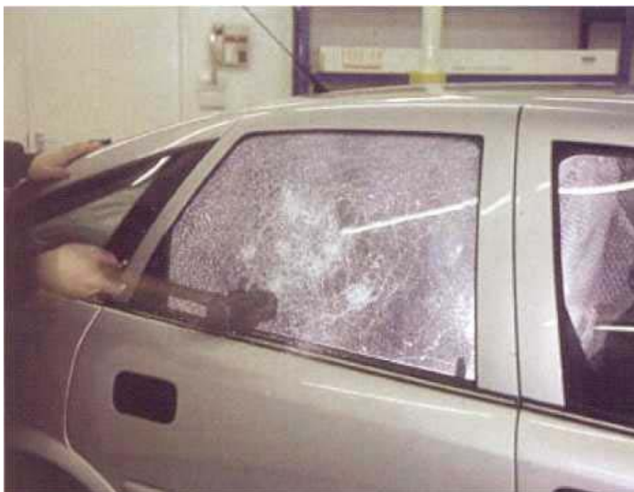
We were understandably reluctant to try the effectiveness of SecureGlass on our 911, but Auto Asylum had recently carried out a demonstration with a Vauxhall Vectra equipped with the safety film. Repeated hits with a club hammer shattered the glass (above), but the safety layer behind (and, sadly, the rest of the car) remained intact
